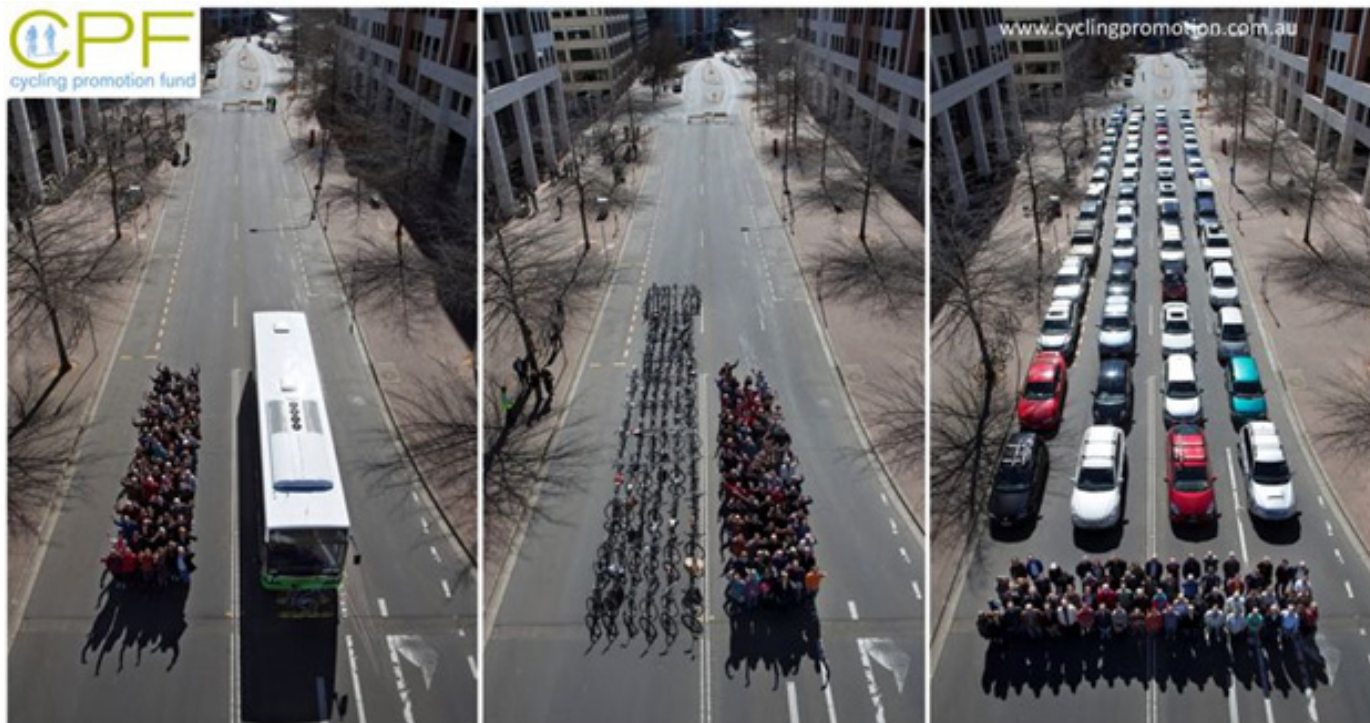
In the leftmost image, one bus carries 44 people in a space about three car lengths. In the rightmost image, 44 cars carry one person each. (Source: Cycling Promotion Fund)
